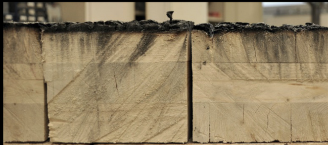
CLT fire testing CREDIT: Naturally Wood BC
