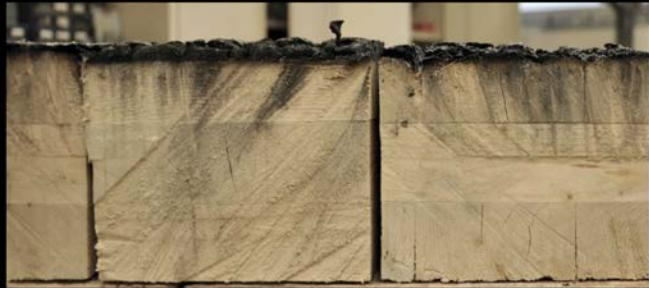
CLT fire testing CREDIT: Naturally Wood BC
